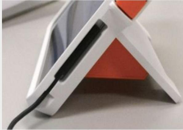
**#2:** Connect the magnetic power supply to the ExpressPoll and plug the power block into an outlet.
